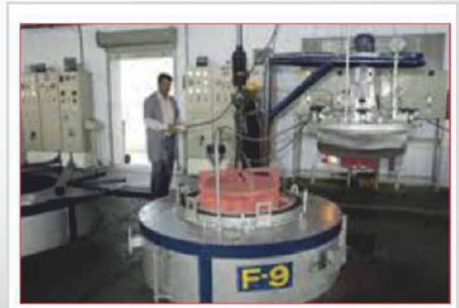
“EN EFF” Gas Carburizing pit furnace
